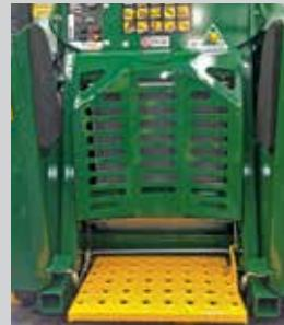
Safety Auxiliary Cut Out - Auxiliary hydraulic flow will neutralize when no operator is present
