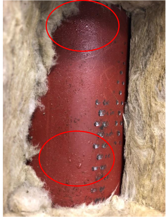
Figure 5 Condensation on the pipe covered with System 2 at the end of the two hours exposure
