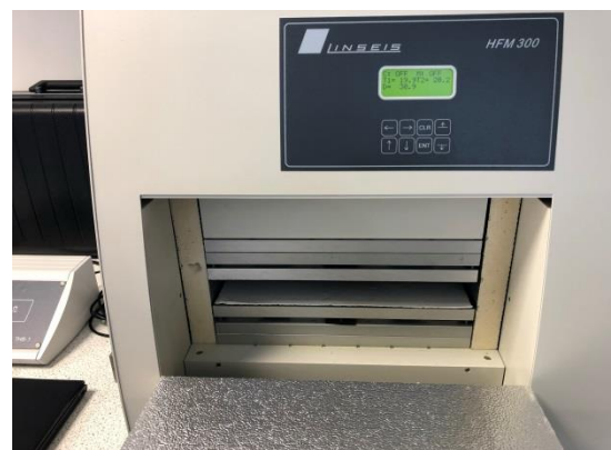
Figure 2 HFM1 heat flow meter
