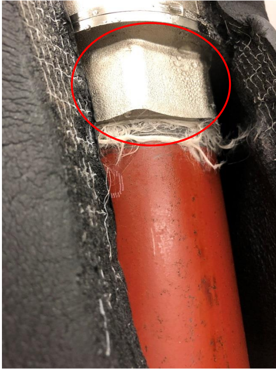
Figure 4 Condensation on the pipe covered with System 1 at the end of the two hours exposure
