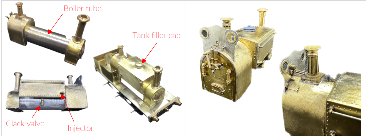
Fig 2.12 – Installing tank & fixtures
