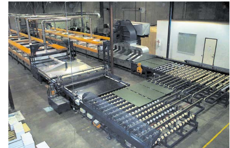
Picture of Contractors Wardrobe®'s Klöpper Mirror Conveyor — located in Sacramento, California. The efficiencies of the line along with the "Copper-Free" chemical solution are environmentally friendly and improve the quality and life of the mirror.
