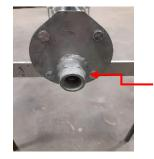
A 1/2" NPT gives the option for a fresh water port at the end of the floor drain to assist with clean out
