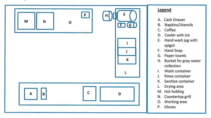
B. Provide a detailed drawing of your floor plan. Show all equipment and utensils, support facilities, and serving areas.
