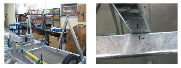
Bolt the "A" frames into position – note that the frames fit on the forward side of the rear crossmember. These are marked with "R" and "L" on both the "A" frame and the rear crossmember to aid assembly
