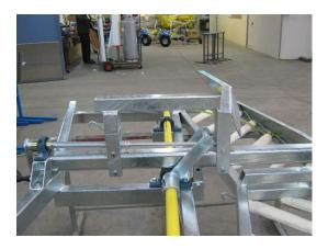
If required, bolt the tank bracket onto the spine making sure there is enough clearance for full travel of the suspension quadrants. See exploded parts diagrams on page 24-27 for details.
