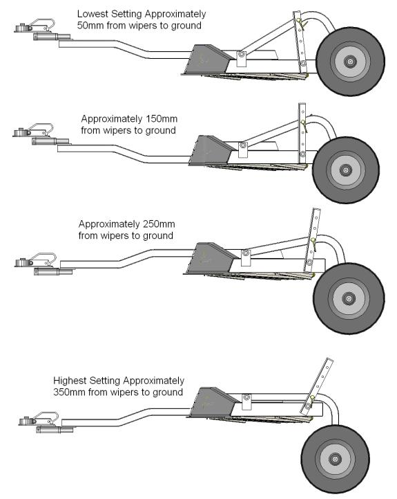
On the Winged Eliminator unit the wings has adjustable skids to match up the height of wings to centre frame to give consistent wiping height.
