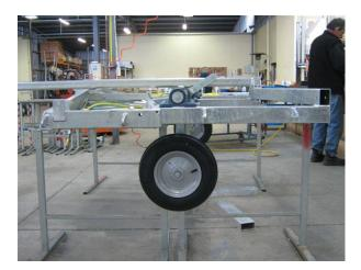
Lower the suspension and fit the wheels
