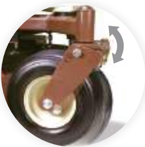
Optional DuraFlex™ Suspension Fork
