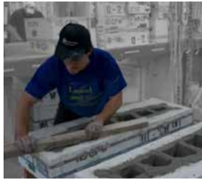
HAND PRESSING TRADITIONAL HAND PRESSING IS THE ORIGINAL MANUFACTURING METHOD OF CASTING ARCHITECTURAL TERRACOTTA. LABOR INTENSIVE PROCESS WHERE CLAY IS PACKED INTO A MULTI-PART MOLD WITH AN OPEN BACK
