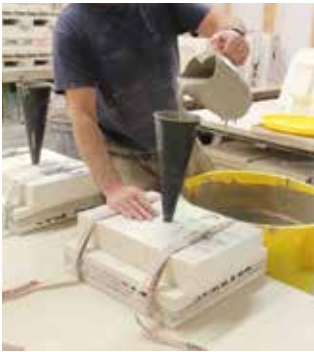
SLIP CAST LIQUID TERRA COTTA IS POURED INTO A PLASTER MOLD. THE PLASTER DRAWS MOISTURE FROM THE LIQUID SLIP. THE EXCESS SLIP IS EVACUATED FROM THE MOLD.
