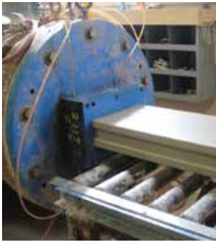
EXTRUSION CLAY IS PUSHED THROUGH A STEEL DIE BY A POWERFUL EXTRUSION AUGER. QUICKEST AND MOST EFFICIENT METHOD OF PRODUCING ARCHITECTURAL TERRA COTTA BUILDING COMPONENTS. IT IS VERY EFFECTIVE FOR PRODUCING A LARGE NUMBER OF BLOCKS WITH THE SAME PROFILE AND LONG CONTINUOUS SPANS OF PANELS.
