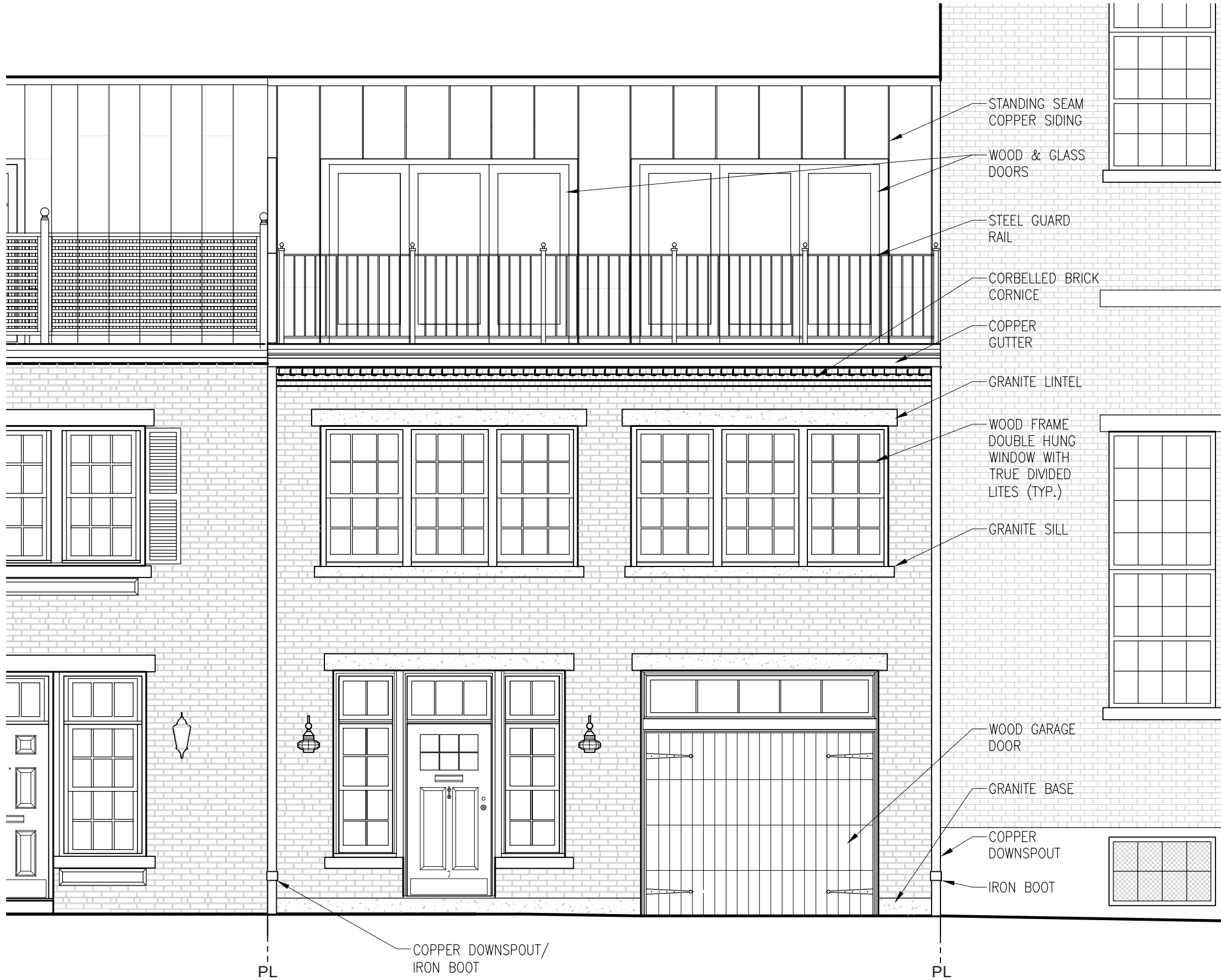
1. PROPOSED ELEVATION SCALE: 1/4" = 1' 0"
