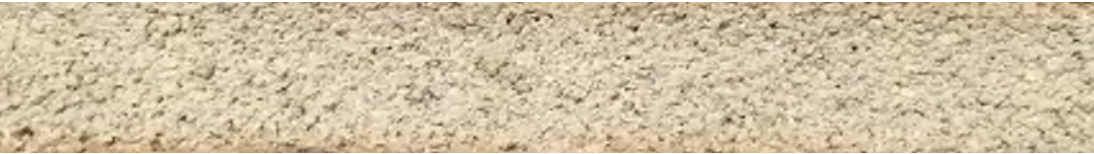
MORTAR TYPE: TYPE N - PORTLAND & LIME MORTAR MORTAR COLOR: SGS 60H WHITE
