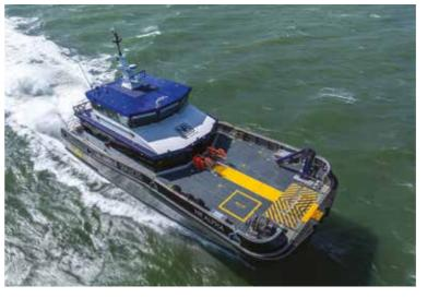
The main deck is 'step free' for the technicians with a large forward deck capable of accommodating 10ft and 20ft containers, main deck crane, pressure washer system and bow transfer area with a cupped Buoyant Works bow fender system to maximise transfer capability. The fuel transfer System has a reel below the main deck to maximise reliability.
