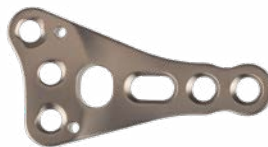
Distal radius plate 3.5 Classic as · Head holes: 3 · Shaft holes: 2 – 13 · Lengths: 42 – 136 mm · Item no. left: 5.877.4X · Item no. right: 5.876.4X · Set Instruments: 19.035.00I
