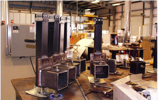
Custom built lifting mechanism built by Clegg Industries -built specifically for the ship move.
