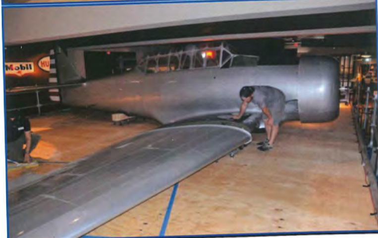
Re-installing wings onto the fuselage
