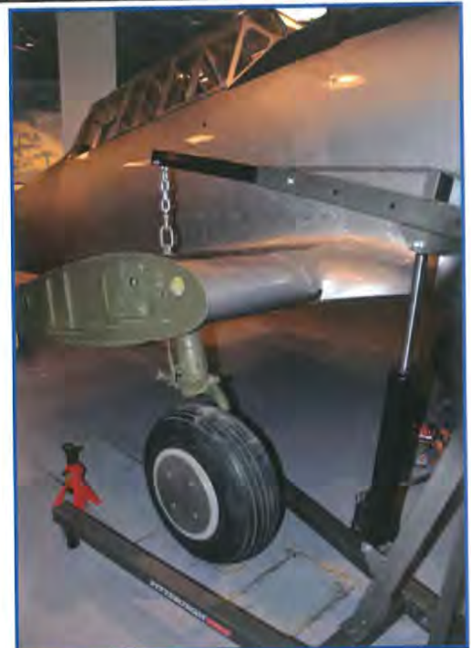
Lifting the aircraft with engine jacks prior to setting cribbing in place
