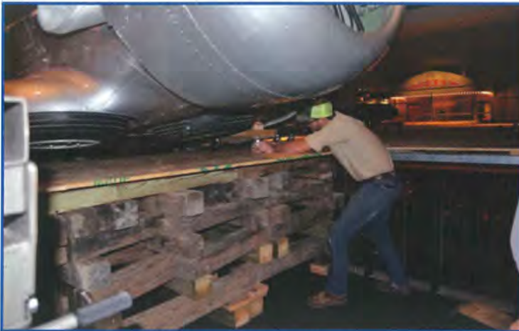
Placing the dollies and fuselage support cradles.
