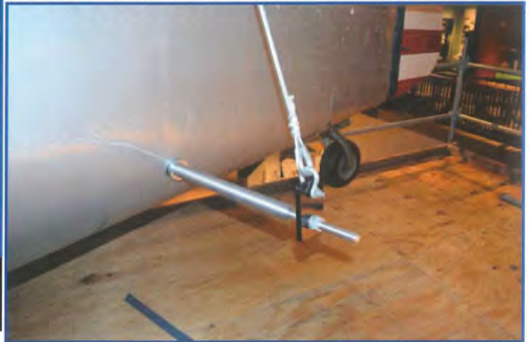
Close up of tail plane rigging; sling attached to lift bar inserted through aircraft lift tube.
