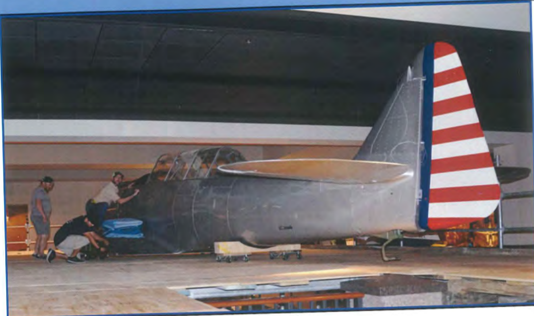
Setting aircraft in position to attach propeller and wings
