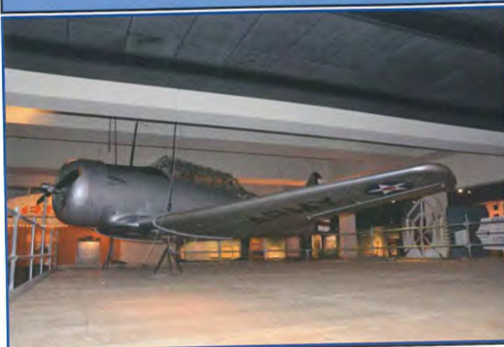
On floor jacks ready for rigging fixtures and cables.
