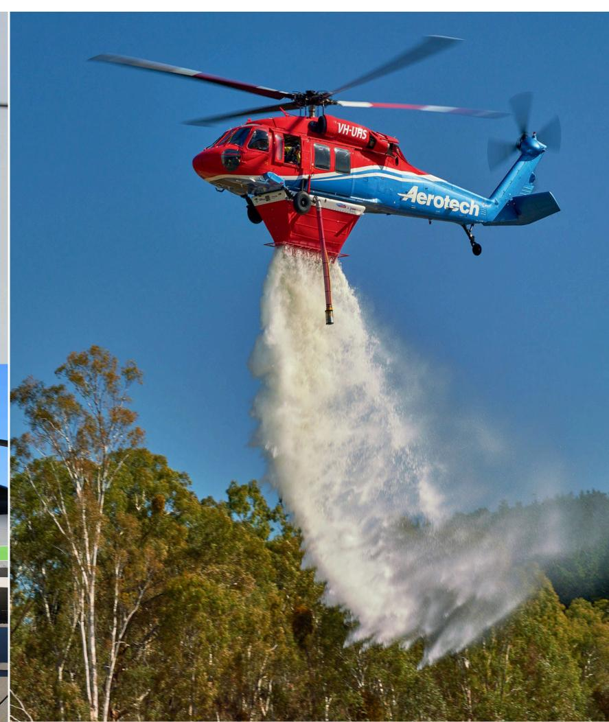
The Helitak FT4500 is approved on the type certificates for the following aircraft models: UH60A, EH60A, H60, HH60A, UH60L, S70, S70C S70A, S70M
