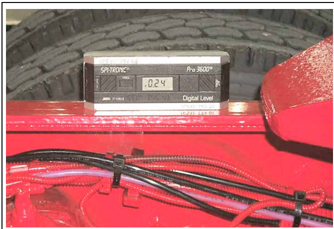
Figure 1-11 Illustration of Inclinometer on the Left-Hand Frame Rail
