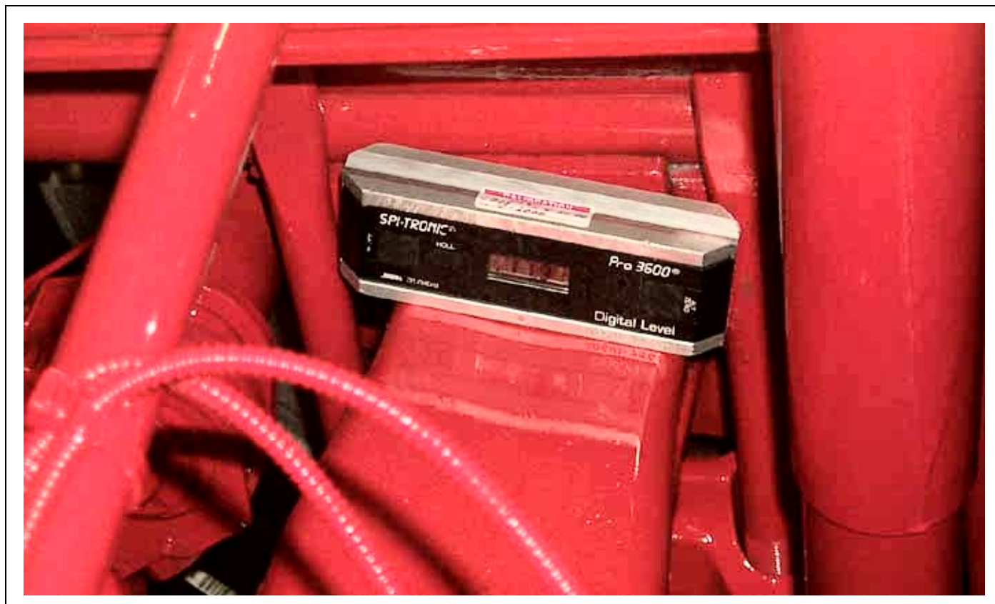
Figure 1-13 Illustration of Using an Inclinometer to Determine Rear-Rear Axle Angle
