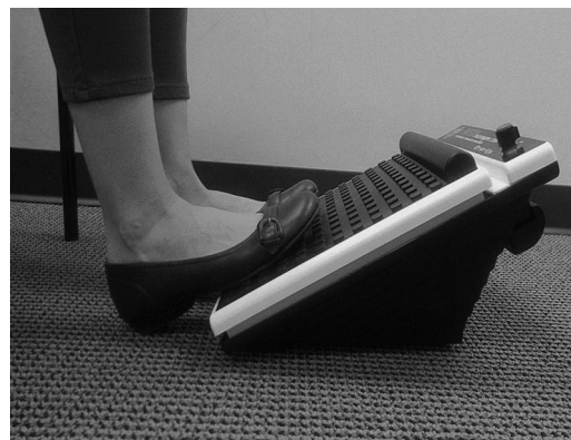
FIGURE 1. Calf muscle pump stimulation device featured in this study (MM-100 Calf Muscle Pump Stimulator, Sonostics, Inc., Vestal, NY), which provides plantar (i.e., sole of the foot) micro-mechanical stimulation through vibration—specifically, a 45 Hz, 50 \mu\text{m} displacement of the frontal portion of the plantar surface.
