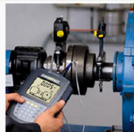
Coupling Shaft Laser alignment
