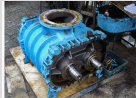
Vacuum Blower Servicing
