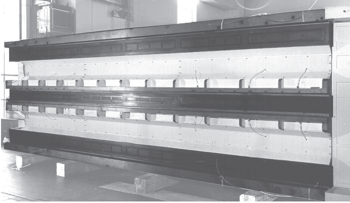
ill. 8: Slide of a grinding machine, hydrostatic guiding system, guiding dimensions 6000 x 230 mm, direct forming-to-size of hydrostatic pockets
