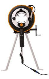
Orbital Services Australia introduces its Orbital Tube Saw. This machine is designed for cutting of thin-walled stainless steel tubes. The cut end face is perpendicular, burr-free and can be directly welded.
