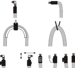
Sharp turns close to the cap during assembly (out of recommended radius) disturbs the structure of PTFE hose has a risk of explosion.
