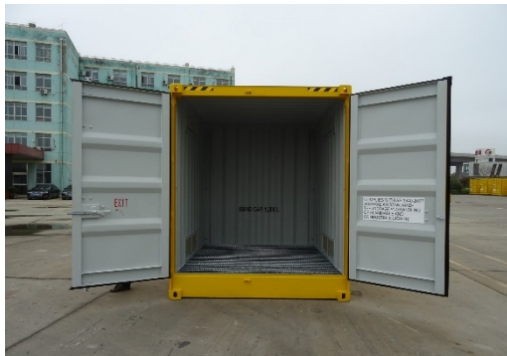
A second bunded 10' container has been delivered to Ramingining to ensure correct storage of waste oil while the primary 10' container is in transit to Darwin.
