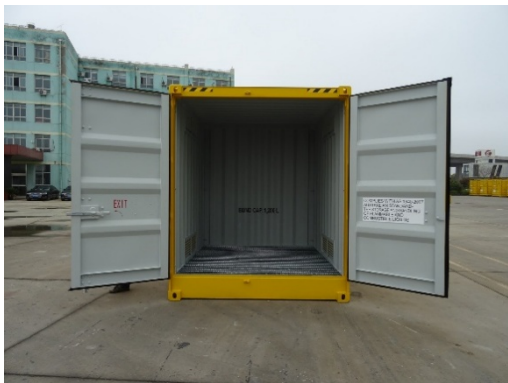
A second bunded 10' container has been delivered to Galiwin'ku to ensure correct storage of waste oil while the primary 10' container is in transit to Darwin.
