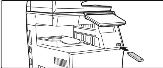
**Connect the USB memory device to the machine.**
