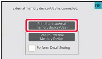
**When a screen for selecting the action appears, tap [Print from external memory device (USB)].**
