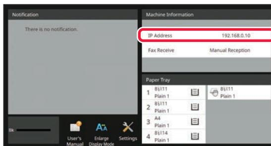
Check the IP address in the machine information.
