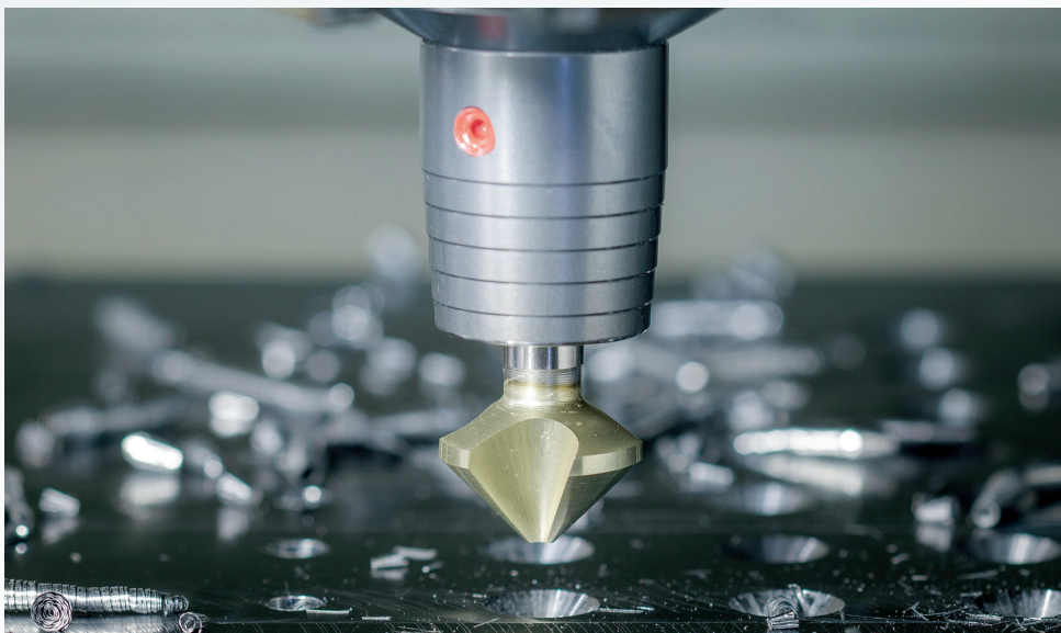
Standard-Senker 42CrMo, v_c = 15 \text{ m/min} , f_u = 0.15
