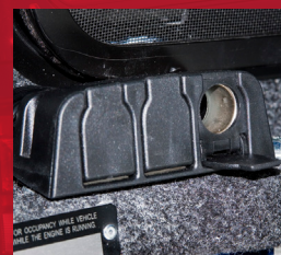
THREE-OUTLET 12- VOLT POWER BLOCK
