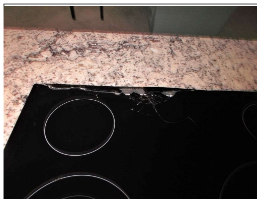
Cook top glass broken
