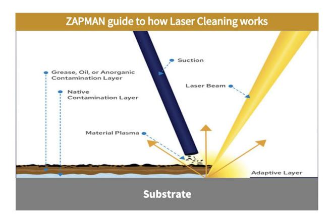
The image above explains the principle of laser cleaning, illustrating how this technology works to remove contaminants from the surface of a material ("substrate").
