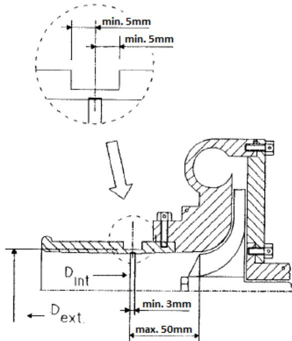
**DRAWING 2: TURBOCHARGER RESTRICTOR ALTERNATE MOUNTING**
