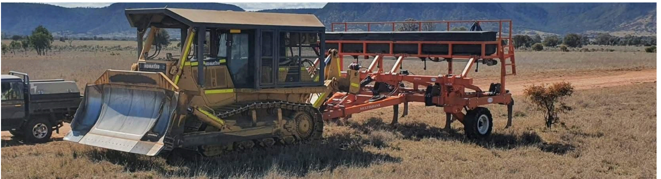
DOZER-DRAWN RIPPER RENOVATING PASTURE COUNTRY
