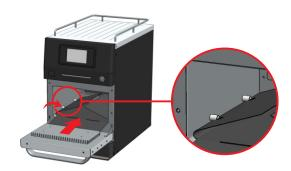
**2-** FOLD SIZE FLAPS AND FIT THE **CAVITY PROTECTION LINER - FIT** INTO THE EQUIPMENT AND THEN SIDE GUIDES AS SHOWN.
