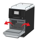
**3-** FULLY OPEN THE **CAVITY PROTECTION LINER** - **FIT** FLAPS, ADJUSTING IT UNTIL IT IS PROPERLY SEATED.
