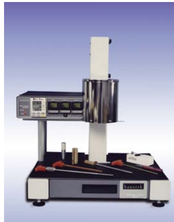
Standard MFI with test and cleaning apparatus.
