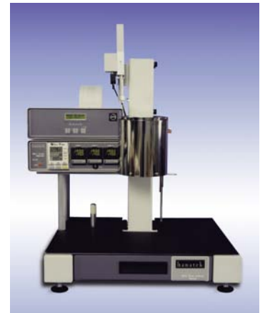
Intermediate MFI with programmable test module.
