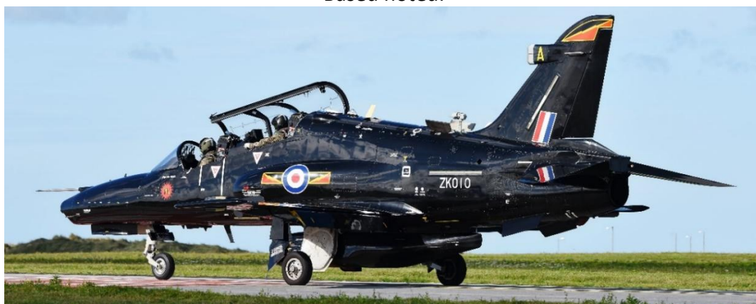
Hawk T.2 ZK010:A 4 Sqn with the RAT [Ram Air Turbine] deployed at the base of the fin.
