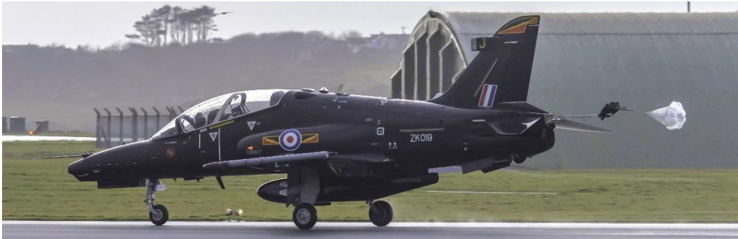
ZK019:J deploying the 'brake chute' on landing.
