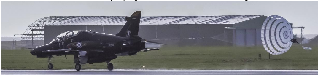
ZK019:J deploying the 'brake chute' on landing.
