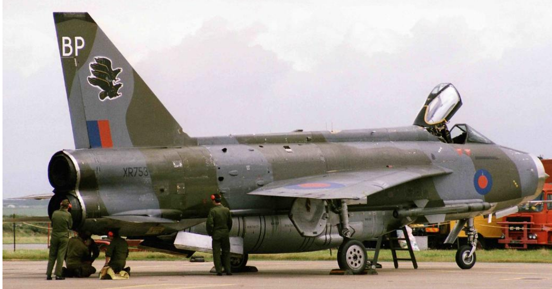
Groundcrew re-pack the brake parachute. [Phil Bradshaw]
