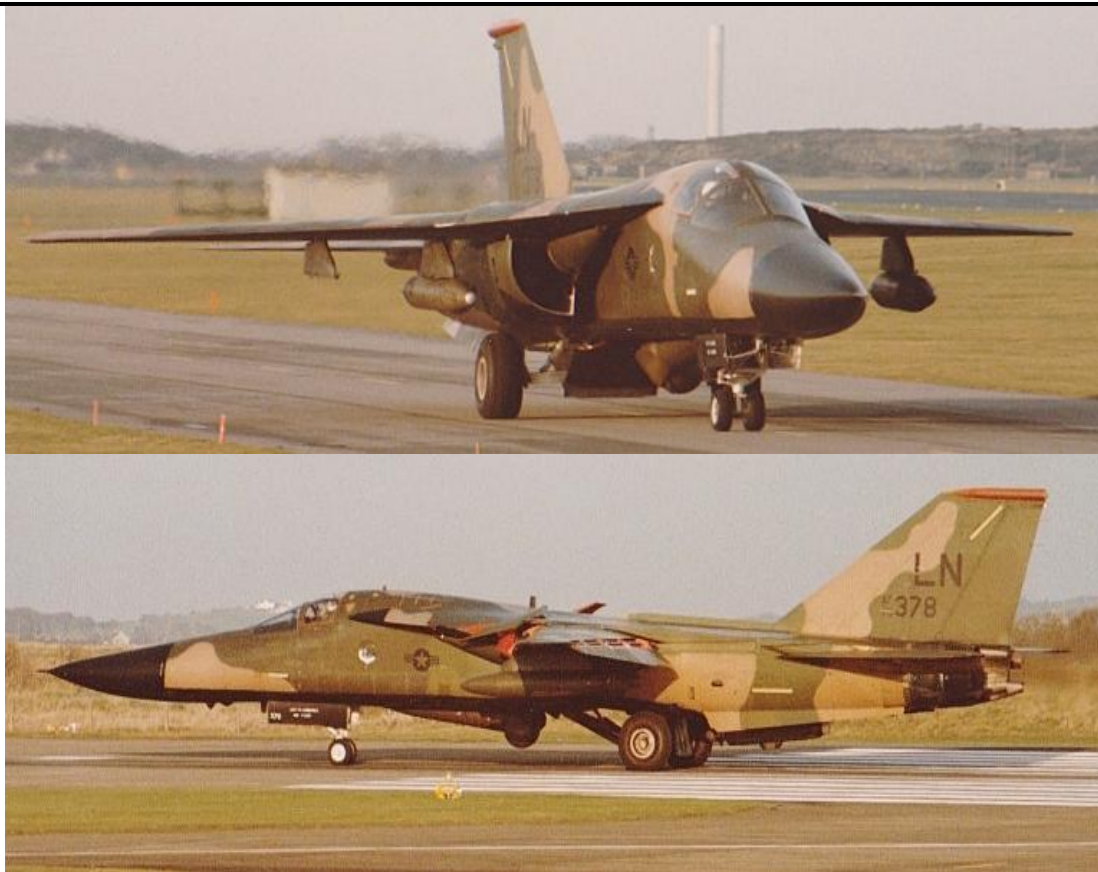
The Pave Tack pod can be seen under the fuselage. [Both: Glyn Jones]
