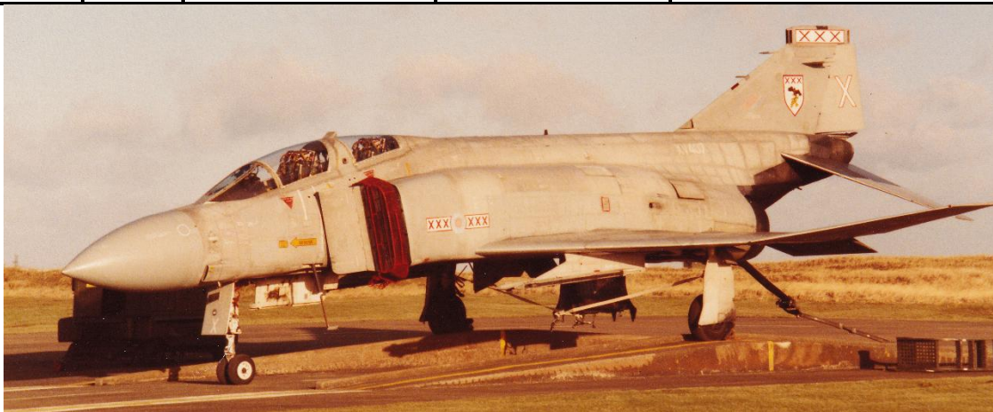
Seen here tethered down ready for a full afterburner engine run. [Hywel Evans]
