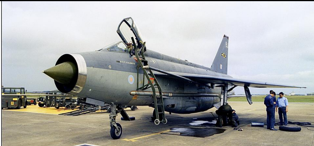
Undergoing a double mainwheel change. [Phil Bradshaw]
