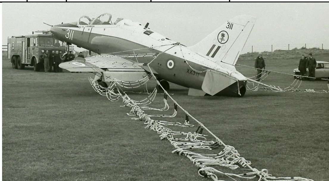
Barrier engagement on Runway 19 after brake failure. Or 10.3 ?
