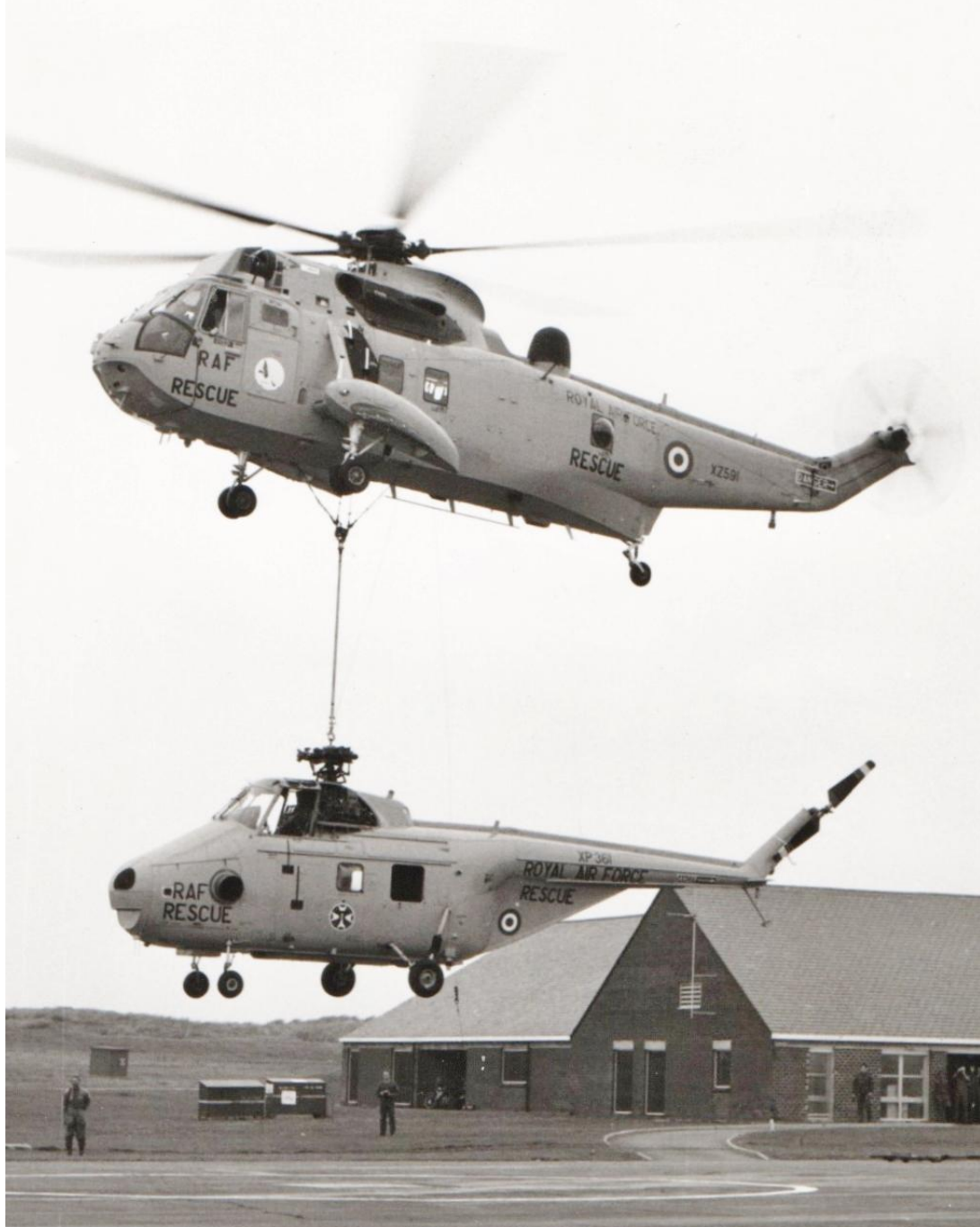
Sea King HAR.3 XZ591 B Flt/202 Sqn [RAF Brawdy] brings XP361 back following its forced landing near Holyhead due to a control restriction during a deck winching exercise. It was recovered from a field on the Eastern side of Holyhead Harbour [5921N 00436W] XP361 was next noted active 15.12.80.
