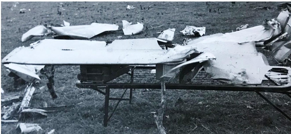
A piece of the canopy can be seen jammed in the tailplane.
