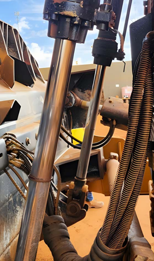
WITHOUT ChromeGuard (Pitted Cylinder Damage)
