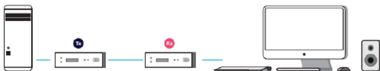
Spot to Spot Mode: Tx – Rx as long distance extension, up to 100m
