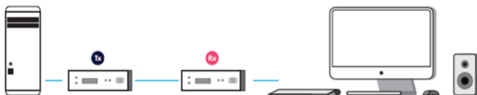
Spot to Spot Mode: Tx – Rx as long distance extension, up to 100m
