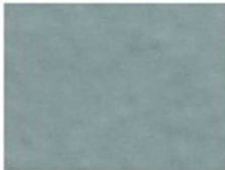
304 Stainless Steel Electropolished Finish 5 - 6 RA
