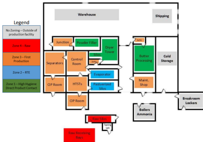
Fig. 4. An example of a Powder and Butter operation with hygiene zoning and hygiene junction rooms/airlocks
