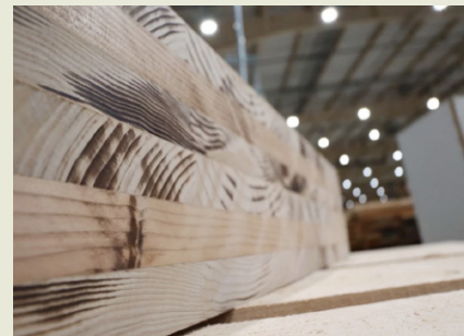
Completed Thermally Modified Advanced Cross Laminated Timber (ACLТ)
