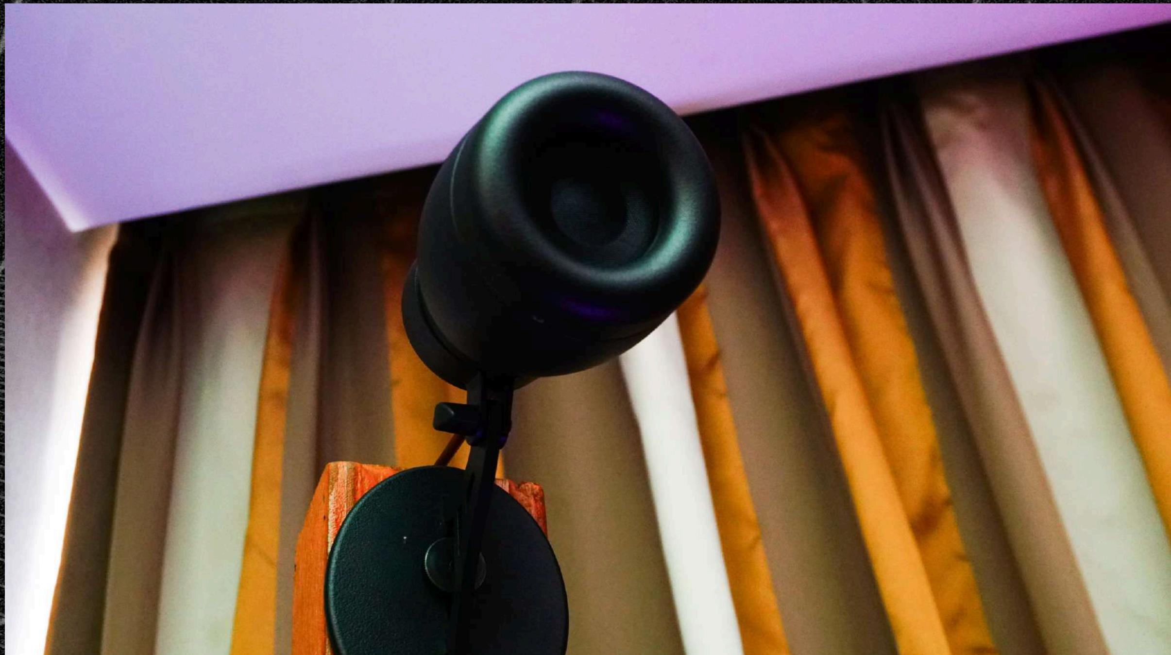
The acoustic excellence is driven by K-array's proprietary, high-efficiency **2-inch transducer**, specifically engineered for this compact series. This design allows the speaker to effortlessly reproduce both speech and music, offering a wide-ranging frequency response and very low distortion. This acoustic versatility establishes the Tornado as a true "**turnkey solution**" for fixed applications requiring both clear voice reproduction and quality background audio.
