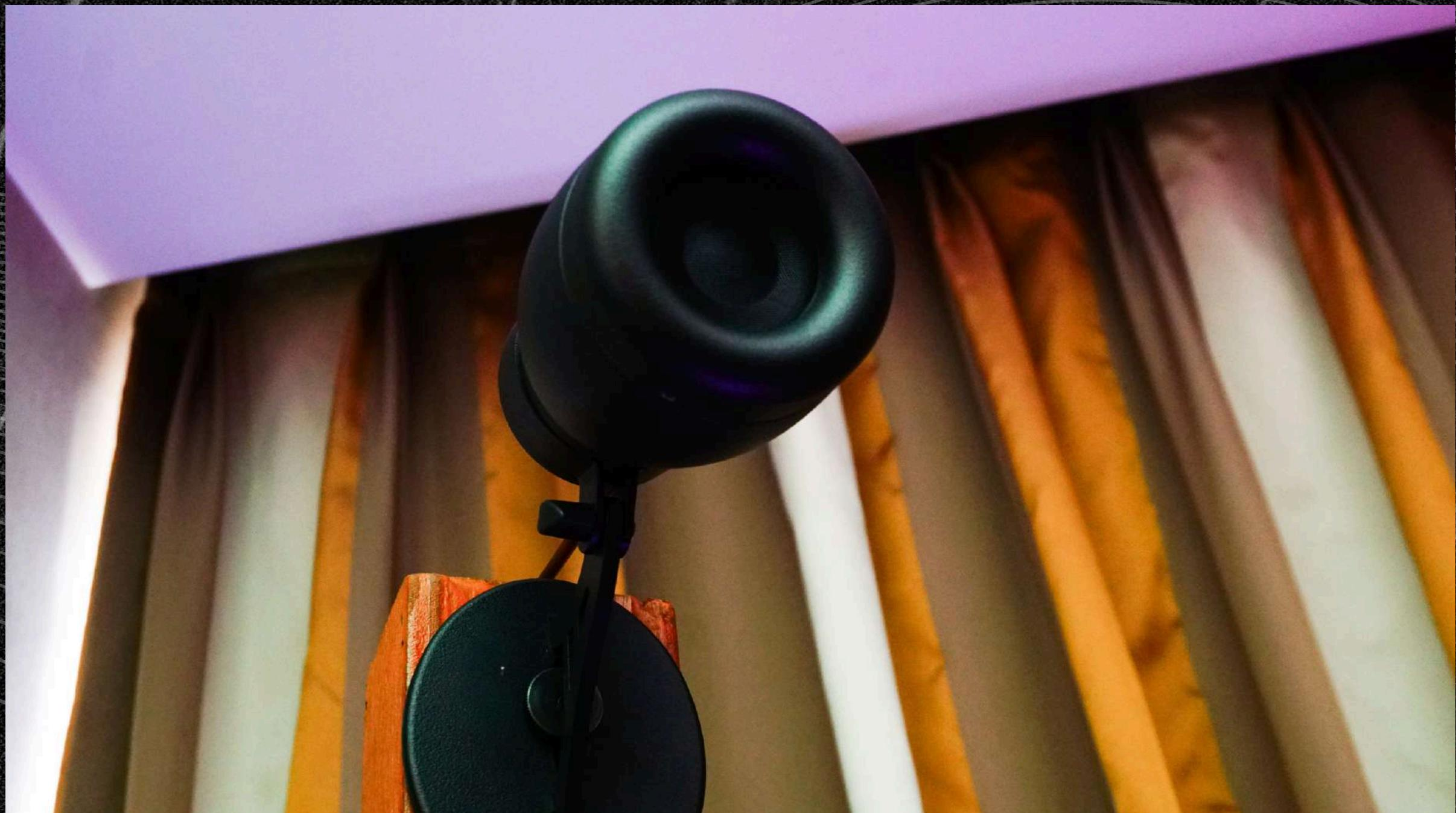
At its core, the Tornado is a **miniature, 2-inch point source speaker** that delivers surprising performance relative to its size. A defining feature is its sophisticated physical construction: the speaker is housed in an **aluminum enclosure meticulously carved from a single metal block**.
