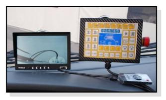
LCD monitor for video camera controlling work area. Next generation digital soft-key keyboard with screen to display work functions and programmes using a CAN-BUS system.
