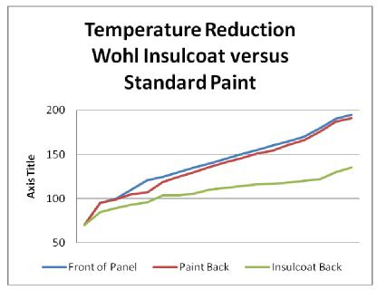
CONCLUSION: When the temperature transmitted through the coating is reduced by 22% the driving force is reduced and the heat transferred is 22% less. The use of Wohl Insulcoat will reduce heat transfer through a metal surface and thereby reduce the heat buildup in a metal building.
