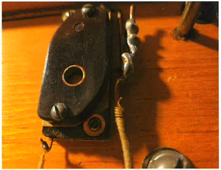
A close up view of an outdated relay switch showing the cotton covered wiring and some soldering.
